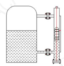
specific value according to the height of the liquid level indicated by the red half reflective column.
